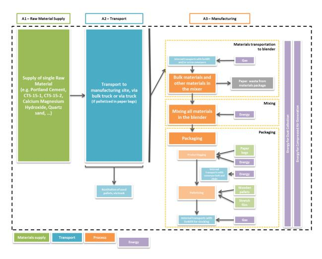
Figure 1: Flow diagram describing the PENETRON products system boundary
